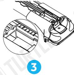
**EN** Adjust the length of the assembled bar to suit the dimension required. Note this may be different for the front and rear of the vehicle.
