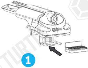
**EN** Attach the gasket that comes out of the box to the metal jaw as shown in the figure.
