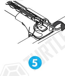
**EN** Using an Allen key, tighten the lateral adjustment screw to lock bars, ensure there is no movement across the width of the vehicle.
