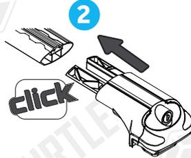
**EN** Insert the lockable feet into each end of the aluminium bar. Ensure the foot is fully inserted until you hear a "click".
