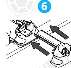
**EN** When you are satisfied with the installation and are happy that all is secure, slide the endcaps onto the bars.
