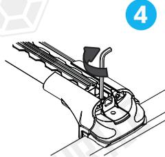
**EN** Place the bars in the desired location of the vehicle. Using an Allen key, tighten the clamp to secure the bar to the roof rails, IMPORTANT! Ensure each foot is mounted correctly on the roof rail.
